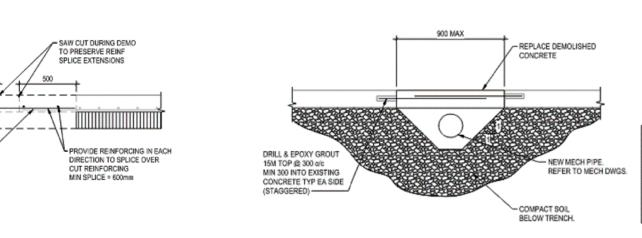
STRUCTURAL SLAB TYPICAL DETAIL AE-202
